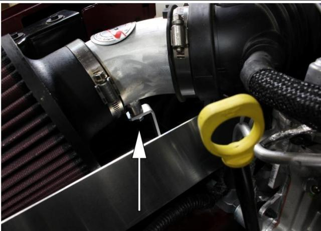
8. Mount the intake pipe onto the intake bracket using the 6mm washer and bolt provided in the hardware kit.
