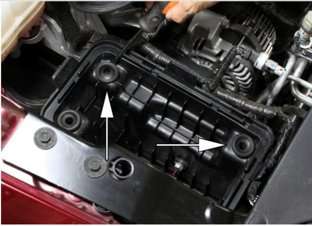
4. Remove the two rubber grommets indicated on the airbox sub assembly.
