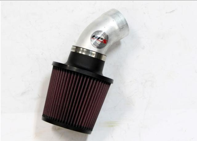
6. Press the HPS air filter onto the HPS intake pipe and tighten the hose clamp.
