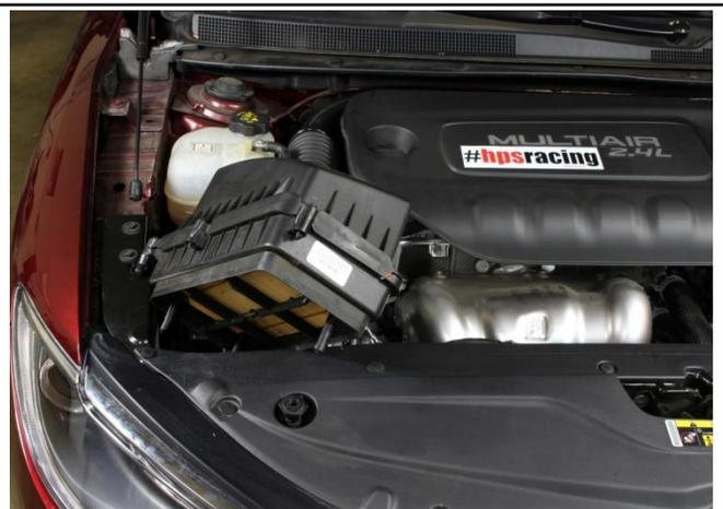
3. Lift up the air box from all 4 corners. There are 4 pegs keeping the air box attached. Remove the assembly from the engine bay.
