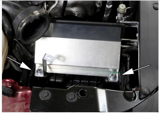
5. Install the HPS heat shield and intake bracket onto the air box sub assembly using an 8mm bolt, 2 washers, and a 8mm nut for each hole.
