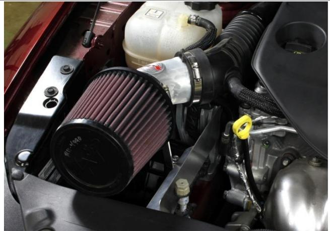
7. Insert the HPS intake pipe into the factory air inlet hose.
