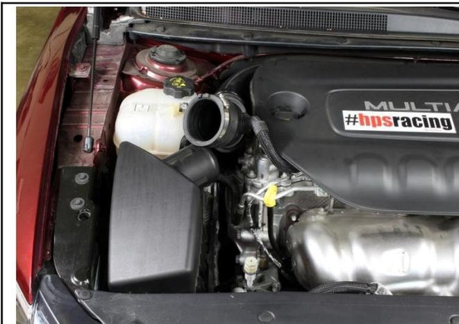
2. Loosen the hose clamp on the intake hose, then detach it from the air box.
