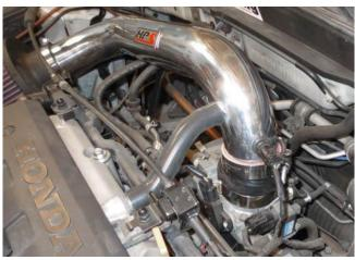
5. Install the 2 1/2" hump coupler and T-bolt clamp onto the throttle body. Position the clamp in a way that it will not impede the throttle cable or any of the sensors. Install the 10mm I.D. grommet into the intake pipe. Place the remaining T-bolt clamp onto the hump coupler and insert the intake pipe into the coupler.
