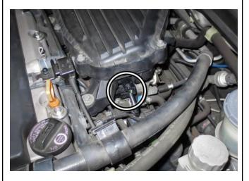
4. Gently pull the intake air temperature (IAT) sensor from the air box. Underneath the IAT port, you should be able to access the clamp that holds the air box to the throttle body. You can use a Phillips (cross) screwdriver to remove it. After this step, you will be able to remove the air box by pulling straight up.
