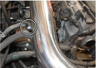
7. Install another 6mm bolt and flat washer to attach the bracket onto the intake pipe.
