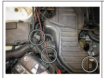
2. Use a 10mm socket with an extension to remove the two bolts on the air resonator and one bolt on the snorkel. Remove the boot from the snorkel to the resonator.
