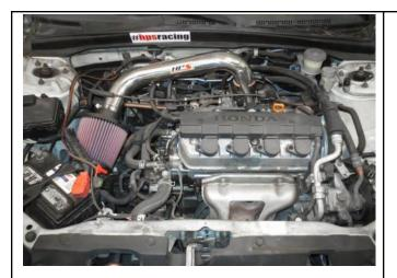
8. Install the HPS air filter and tighten the clamp with a flat head (blade) screwdriver. Install the included vacuum hose onto the valve cover and connect it to the intake. Trimming may be required if the hose is too long.
